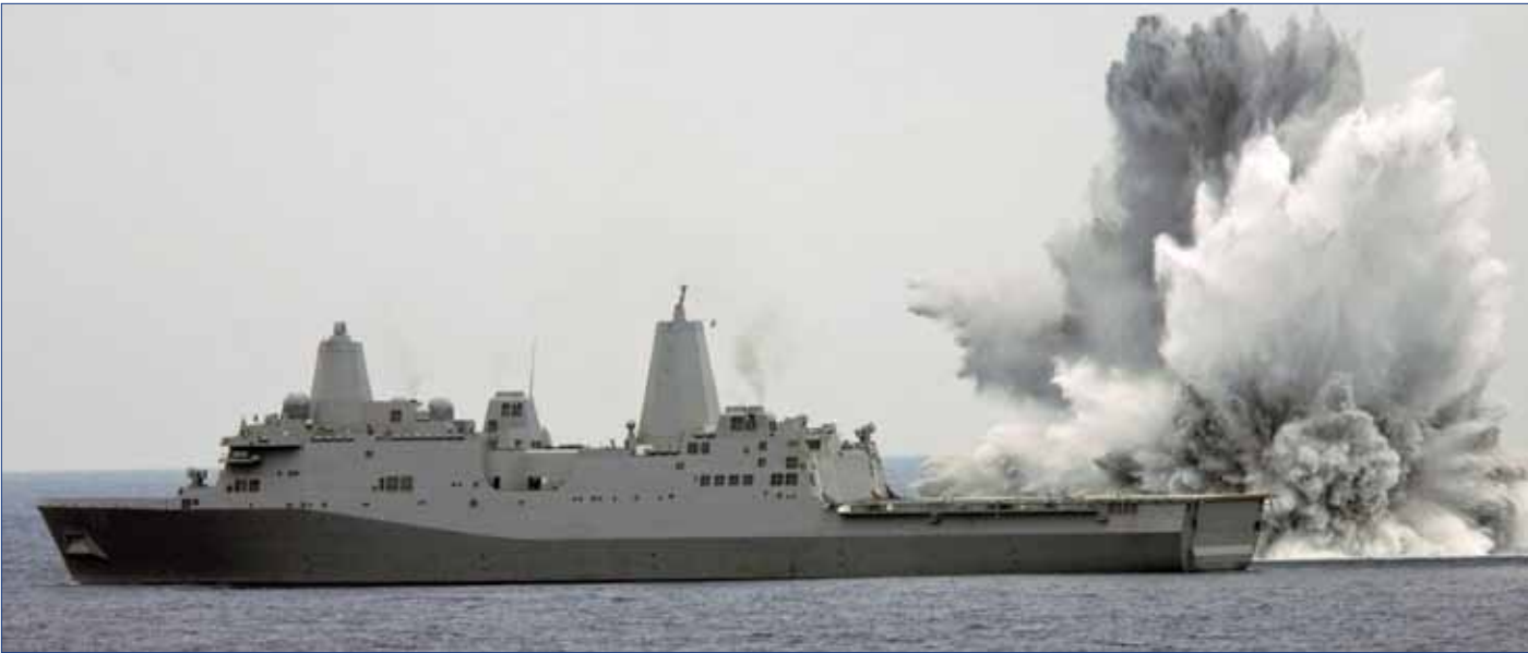
▲ A 10,000-pound underwater explosion rocks USS Mesa Verde (LPD 19) during a shock test off the Florida coast.
